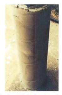
Simulated blocked perforated casing target before pulsing
