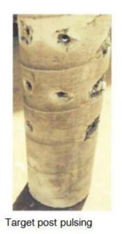
Fig. 4. Effect of PPT on the cement integrity after and before its application.<sup>1</sup>
