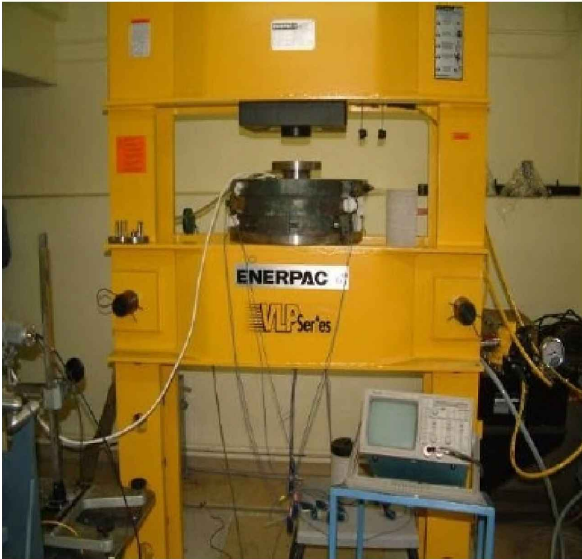
Figure 1.2. Hydraulic frame hosting the triaxial cell
