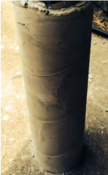
Simulated blocked perforated casing Target Before Pulsing
