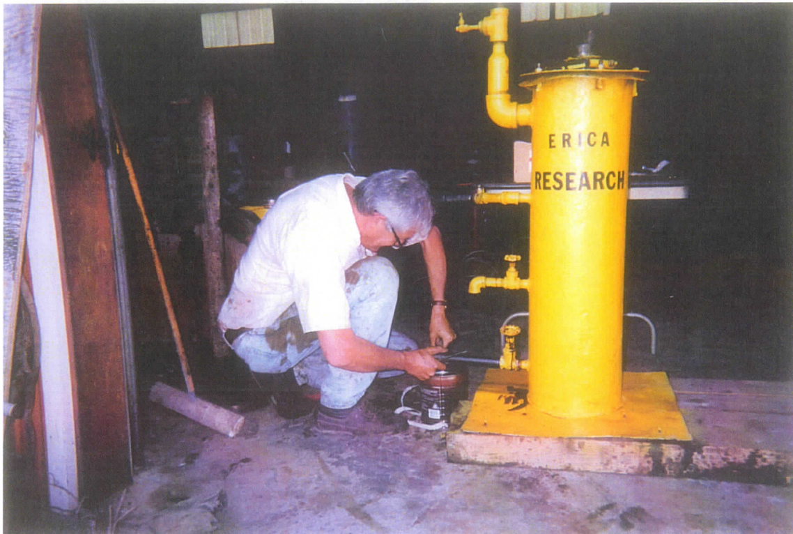
CIRCULATION TEST UNIT TO TEST VISCOSITY
