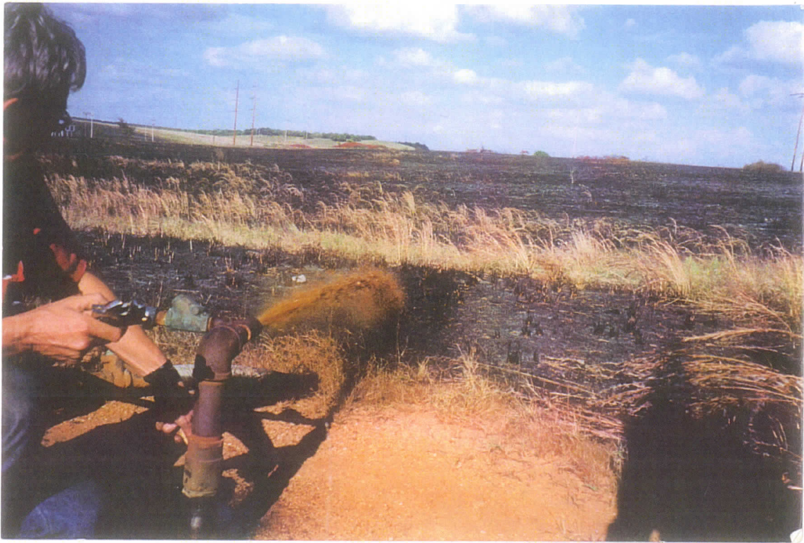
THIS WELL WAS NOT PRODUCING AND ONLY HAD A VALVE, NO PUMP JACK. THIS WELL WAS 1,320 FEET FROM THE OSAGE TEST WELL. NOTICE THE GASOUS OIL FLOWING WHEN THE VALVE WAS OPENED.
