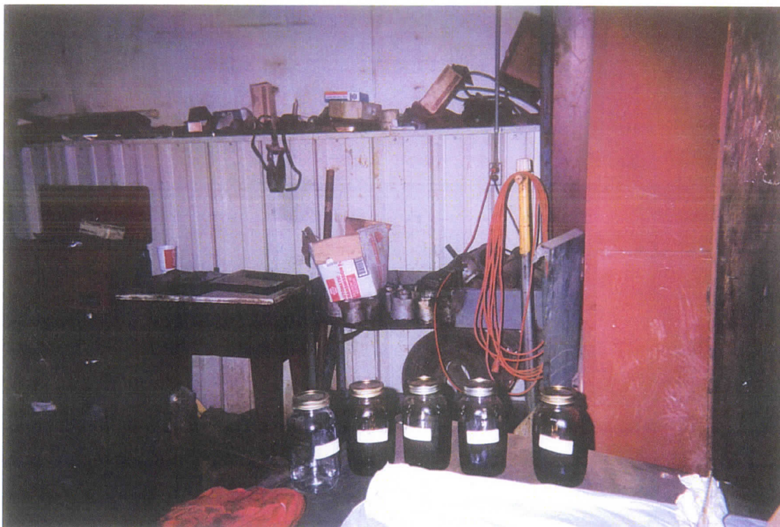
CRUDE OIL SAMPLES WITH NUMBER OF SHOTS TO BE TESTED FOR VISCOSITY
